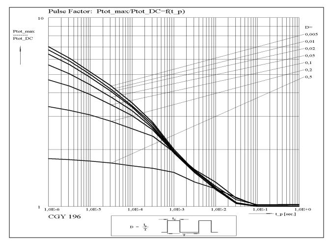
$\mathsf{P}_{\text{tot-max}}$  should not exceed the absolute maximum rating for the dissipated power  $\mathsf{P}_{\mathsf{Pulse}}$  = "Pulse peak power" = 2 W
