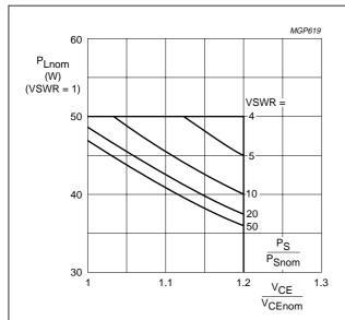
Fig.11 R.F. SOAR; (short-time operation during mismatch); f = 175 MHz;  $T_h$  = 70 °C;  $R_{th\ mb-h}$  = 0,3 K/W;  $V_{CEnom}$  = 12,5 V or 13,5 V;  $P_S$  =  $P_{Snom}$  at  $V_{CEnom}$  and VSWR =1 measured in the circuit of Fig.7.
