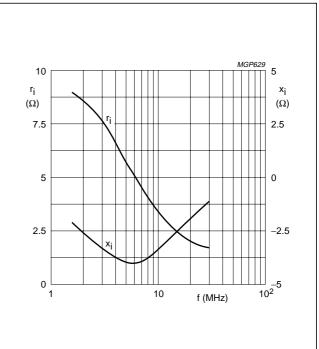
Fig.21 Input impedance (series components) as a function of frequency.
