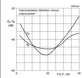
$V_{CE}$  = 13,5 V;  $f_1$  = 28,000 MHz;  $f_2$  = 28,001 MHz;  $T_h$  = 25 °C;  $R_{th\;mb\text{-}h} \le$  0,3 K/W ;  $I_{C(ZS)}$  = 25 mA; typical values.
